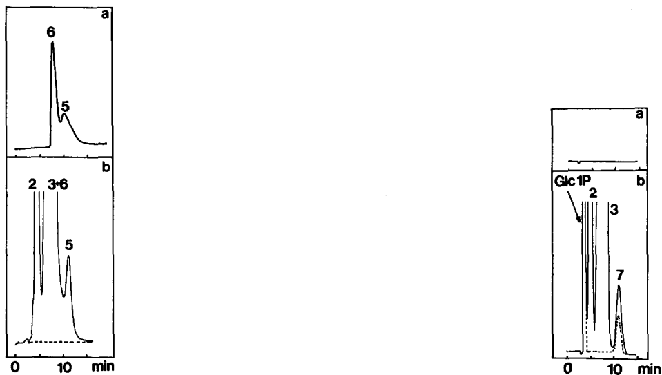
Fig. 6. Elution profiles for adenosine phosphorylated by diphosphonate (3) at pH 10 and 20°C for 30 min. 2 = Phosphonate; 5 = adenosine 2'-H-phosphonate; 6 = adenosine 3'-H-phosphonate. Adenosine has disappeared after 30-min incubation with diphosphonate. Eluent: 0.15 M KCl + 0.1% Na 4 EDTA. Wavelength and meaning of the solid and the dotted lines in (b) as in Fig. 4. Peak numbers correspond to the compound numbers in Fig. 1.
