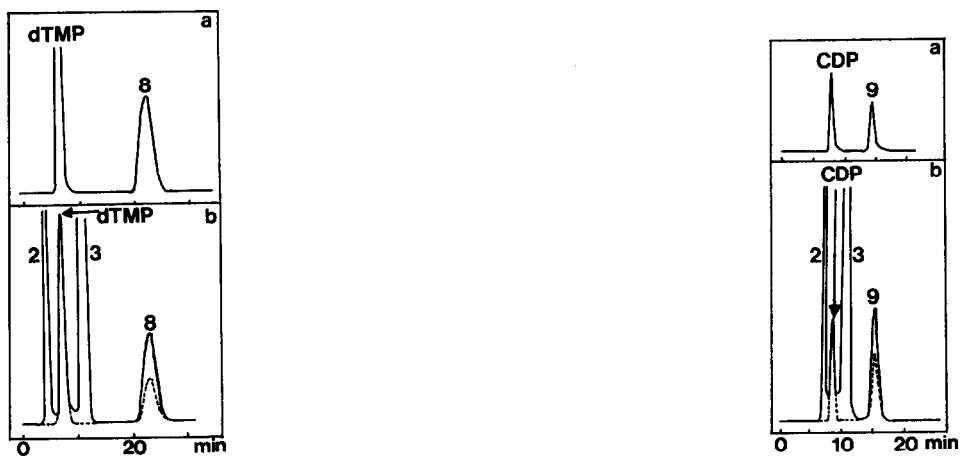
Fig. 8. Elution profiles for thymidine 5'-monophosphate (dTMP) phosphonylated by diphosphonate ( 3 ) at pH 6 and 80°C for 4 h. 2 = Phosphonate; 8 = phosphonylated dTMP. Eluent: 0.2 M KCl + 0.1% Na 4 EDTA. Wavelength and meaning of the solid and the dotted lines in (b) as in Fig. 4. Peak numbers correspond to the compound numbers in Fig. 1.
